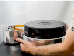
**Step 5**: position the belt along the platter's circumference at the approximate height of the pulley. Proceed around the perimeter of the platter to move the belt into position.
