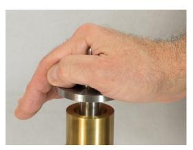
d) As you continue to press the spindle down, you will feel an increase in resistance when the spindle contacts the pool of oil at the bottom.
